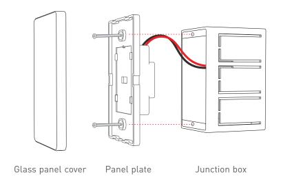
Step 4: Put the panel cover in place. Gently snap the panel cover onto the plate.
