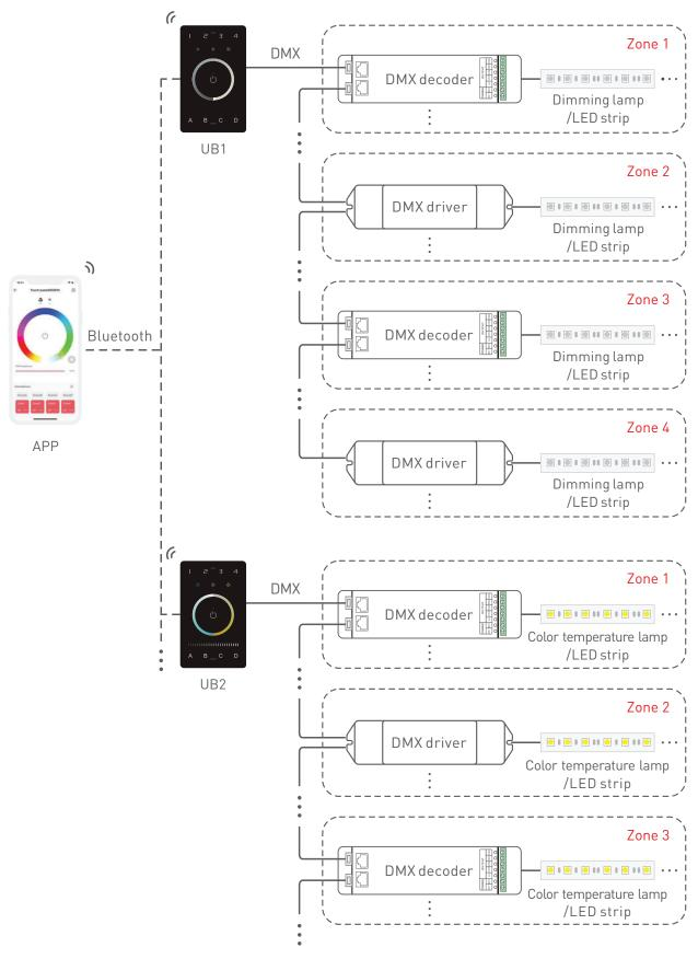
Each zone can be installed with multiple decoders. When the total number of decoders in 4 zones exceeds 32, please add DMX signal amplifiers.
