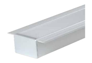
profile designed for mud-in applications and compatible with LED strips up to 37.5mm (1.47") wide. Made from high quality extrusions aluminum, these provide superior thermal management for LED strips prolonging the lighting system's lifespan. It is manufactured with a patented frosted diffuser for maximum lumen output and wider beam distribution.
