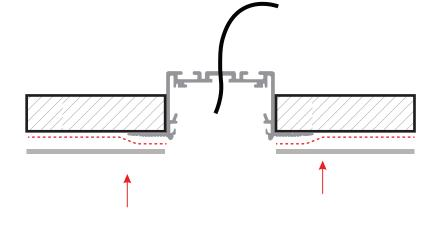
Mount LED strip. Lay strip carefully onto profile making sure the full length has adhered properly and flat onto the profile. Then attach the lens
