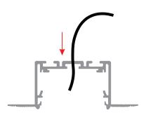
Attach the fixture to the installation surface by securing it onto place with screws on either side. Make sure to use the appropriate screws for metal applications.
