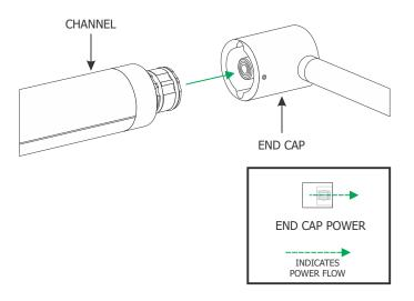
1: Align the channel with the stem end cap and slide into place.
