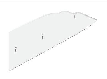
RUN WIRES THROUGH HOLES INTO PROFILE, THEN POSITION PROFILE ON THE CEILING. SCREW THE PROFILE SECURELY ONTO THE CEILING, THEN CONNECT WIRE TO POWER SUPPLY.
