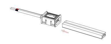
Press cap onto holes to have the copper of the connector connected to the LED tape's circuit. The connection is successful once you hear a click.
