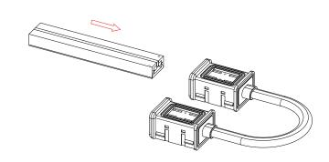
Press cap onto holes to have the copper of the connector connected to the LED tape's circuit. The connection is successful once you hear a click.
