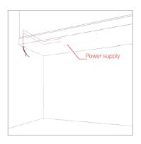
Make the electrical connection to the power supply and then run the wires to the location of the light fixtures.
