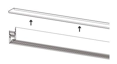
Peel off adhesive backing on LED strip and mount onto aluminum profile, making sure that the whole length of the strip is pressed firmly to adhere properly.
