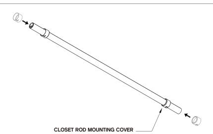
INSTALL ONTO CLOSET ROD MOUNTING BASE SUPPORT.
