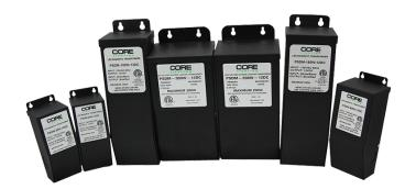
PSDM-150W-12V is a constant voltage LED driver equipped with a magnetic transformer core. It features built-in protection for both the load and the driver via auto-reset breakers (one on the input and one on the output). Its durable, coated metal box includes 2 knock-outs, one on each side, for easy installation that complies with electrical code standards. Compatible with any standard MLV/incandescent TRIAC (leading edge) dimmer switch.
