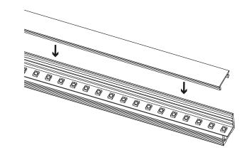
3 MOUNT END CAPS. FOR LEAD WIRE GOING THROUGH THE END OF THE PROFILE, RUN LEAD WIRE THROUGH END CAP WITH HOLE. USE AN END CAP WITHOUT A HOLE FOR LEAD WIRES GOING THROUG BOTTOM OF PROFILE.
