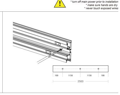
5 Place insulation on both ends of LED strip and attach to carrier. Connect rigid modular to pins correctly (do not confuse anode with cathode), then slide the rigid module into carrier.
