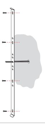
Connect the wires, align the fixture with the mounting bracket and secure with two set screws on top and bottom of the fixture.
