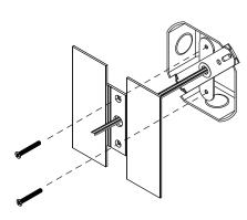
Align the bracket to the gap on the wall plate /canopy kit then mount the bracket using the screws provided. Secure the bracket tightly.
