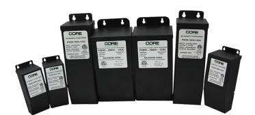
**PSDM-60W-12V** is a constant voltage Class 2 LED driver equipped with a magnetic transformer core. It features built-in protection for both the load and the driver via auto-reset breakers (one on the input and one on the output). Its durable, coated metal box includes 2 knock-outs, one on each side, for easy installation that complies with electrical code standards. Compatible with any standard MLV/incandescent TRIAC (leading edge) dimmer switch.
