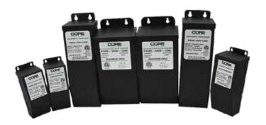
**PSDM-40W-12V** is a constant voltage Class 2 LED driver equipped with a magnetic transformer core. It features built-in protection for both the load and the driver via auto-reset breakers (one on the input and one on the output). Its durable, coated metal box includes 2 knock-outs, one on each side, for easy installation that complies with electrical code standards. Compatible with any standard MLV/incandescent TRIAC (leading edge) dimmer switch.
