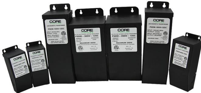
**PSDM-300W-12V** is a constant voltage LED driver equipped with a magnetic transformer core. It features built-in protection for both the load and the driver via auto-reset breakers (one on the input and one on the output). Its durable, coated metal box includes knock-outs for easy installation that complies with electrical code standards. Compatible with any standard MLV/incandescent TRIAC (leading edge) dimmer switch.
