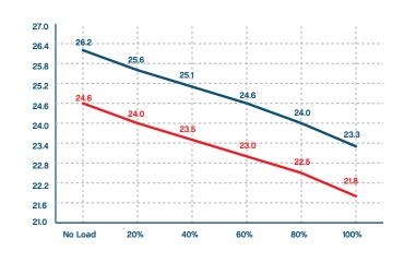
OUTPUT VOLTAGE VS. LOAD
