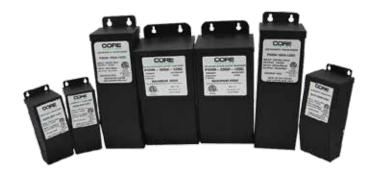
**PSDM-150W-24V** is a constant voltage LED driver equipped with a magnetic transformer core. It features built-in protection for both the load and the driver via auto-reset breakers (one on the input and one on the output). Its durable, coated metal box includes 4 knock-outs for easy installation that complies with electrical code standards. Compatible with any standard MLV/incandescent TRIAC (leading edge) dimmer switch.
