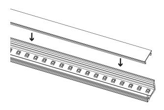
MOUNT END CAPS. FOR LEAD WIRE GOING THROUGH THE END OF THE PROFILE, RUN LEAD WIRE THROUGH END CAP WITH HOLE. USE AN END CAP WITHOUT A HOLE FOR LEAD WIRES GOING THROUG BOTTOM OF PROFILE.
