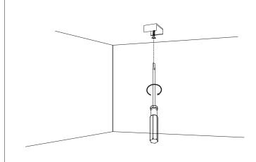
MAKE NECESSARY WIRE CONNECTIONS. MAKE SURE TO FOLLOW WIRING DIAGRAM OF POWER SUPPLY, DIMMER ETC... FIX PROFILE INTO POSITION AND ATTACH TO MOUNTING CLIPS. FIXTURE WILL SNAP SECURELY ONTO MOUNTING CLIPS WHEN PROPERLY FASTENED.
