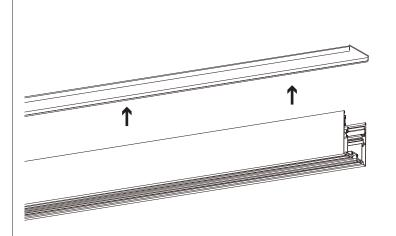
MAKE A SLOT THE SAME SIZE AS THE PROFILE ON THE CEILING TO ACCOMODATE CHANNEL
