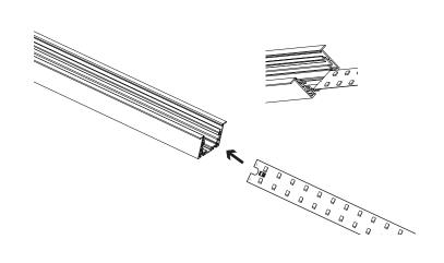
6 INSTALL DIFFUSER ONTO PROFILE
