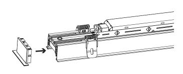
9 CONNECT POWER SUPPLY TO WIRE IN CEILING THEN INSTALL PROFILE INTO SLOT.
