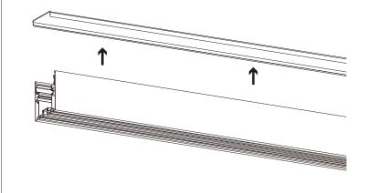
**3** Peel off adhesive backing on LED strip and mount onto aluminum profile, making sure that the whole length of the strip is pressed firmly to adhere properly.
