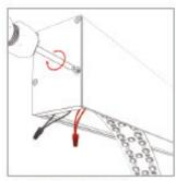
5. Secure the end caps and install the LED strip on to the fixture surface
